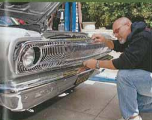
In 1965, Coronets came with quad headlights. A-990 cars did not and required the melding of multiple grilles. The headlight grille is one of the signature visual items on a '65 A-990 Dodge.
