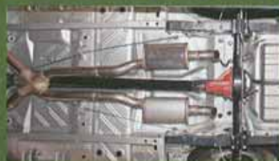
Like the rest of the car, the exhaust installation is simple but elegant. The relocated rear springs and large-diameter exhaust pipes prevent the installation of rear exiting pipes.
